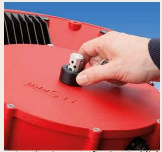
Pass the cable through the opening with the recess - Attach the angle coupling to the connector - Place the strain relief ball in the recess - DONE.
